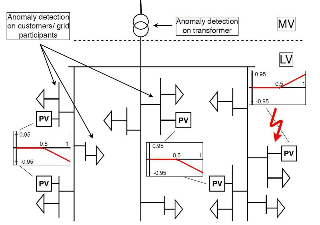
Set-up for anomalies to be detected in a power grid
